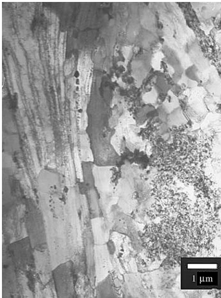
Fig. 12. TEM image of 1% \text{Y}_2\text{O}_3 ODS steel elaborated from EUROFER + \text{Y}_2\text{O}_3 powders mixed by attritor milling in the same condition that the one presented in Fig. 10(d). The nano-sized grains ( \sim 200\text{nm} ) are visible on the bottom right corner.
